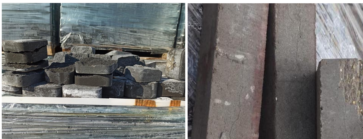
Figure 7 - Fault due to incorrect humidity.
