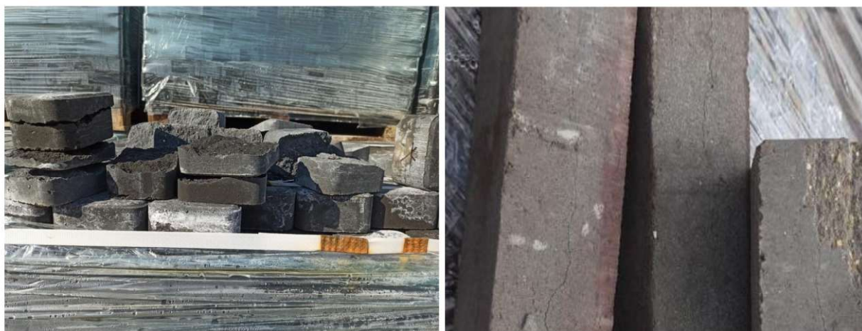
Figure 7 - Fault due to incorrect humidity.
