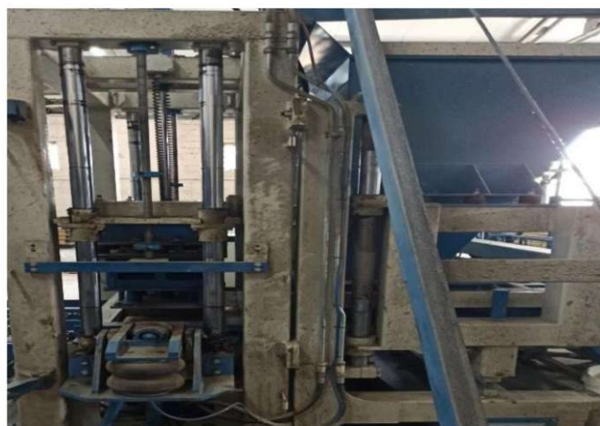
Figure 3 - Automatic trolley-type vibrating machine
